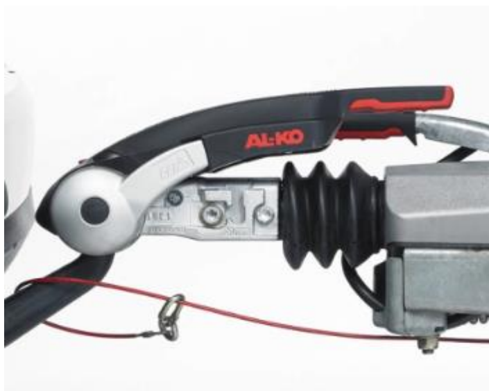
Figure 2 – Method of attaching the breakaway cable to a detachable towball
