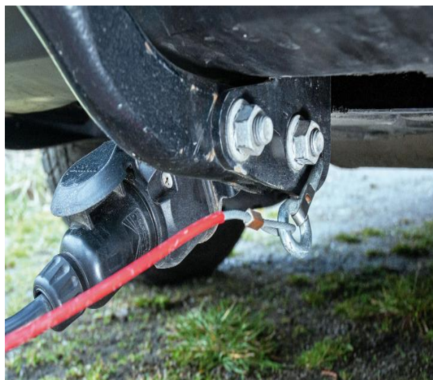
Figure 1 – Method of attaching the breakaway cable to a fixed towball
