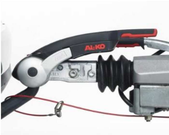
Figure 1- Method of attachment of the breakaway cable- fixed tow hitch
