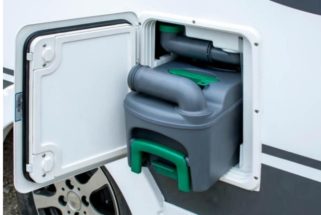
Figure 6- ejected toilet cassette visible through the open access door
