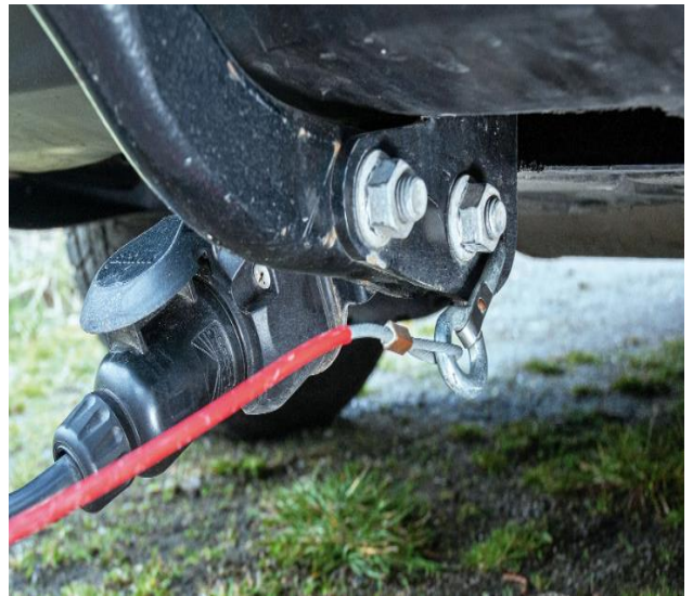
Figure 2-Method of attachment of the breakaway cable – removable tow hitch
